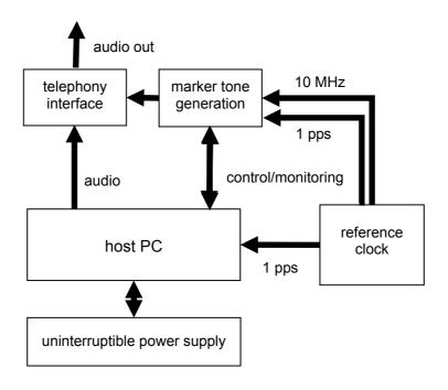
Figure 2: The NMI speaking clock system.
