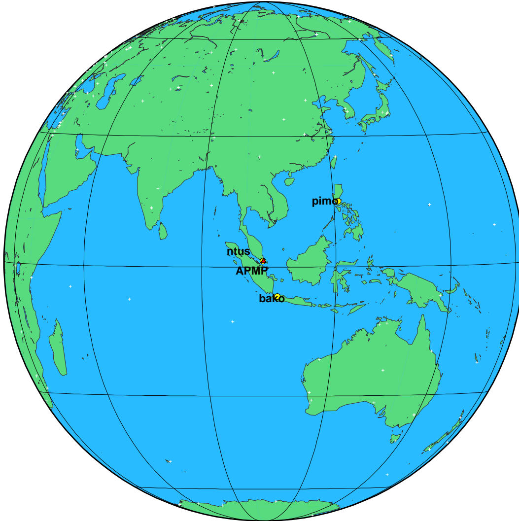
Figure 1: Global View – submitted GPS station(s) and nearby IGS GPS stations used in the processing; triangle(s) represent submitted user data; circle(s) represent the nearest available IGS stations.
