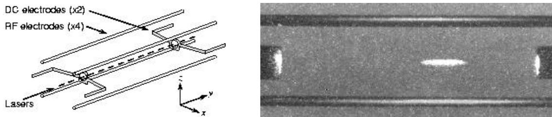
Figure 1: (Left) Electrode configuration of the linear trap. We refer to motion in the  $y$  direction as axial, and in the  $x$ - $z$  plane as transverse. (Right) The laser-cooled ion cloud, approximately 10 mm long with a radius of 1.5 mm. RF electrodes are visible top and bottom (diameter 2.3 mm, separation 20 mm) and DC electrodes left and right (separation 60 mm).
