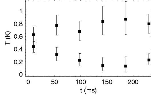
Figure 6: Upper and lower traces show temperature  $T$  obtained from half-profiles above and below line centre varying with time  $t$  after shutter opens.
