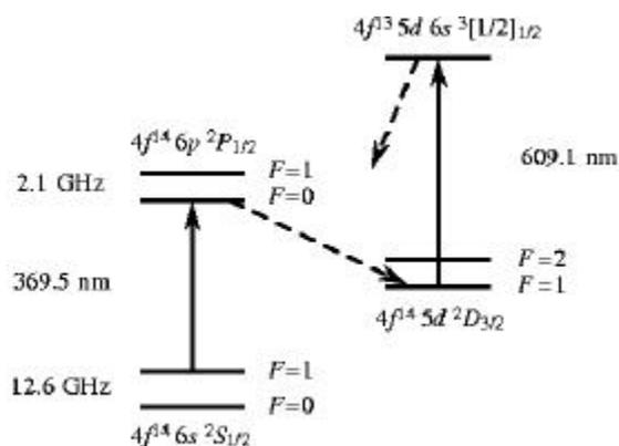
Figure 2: Partial energy level diagram of the  $^{171}\text{Yb}^+$  ion.
