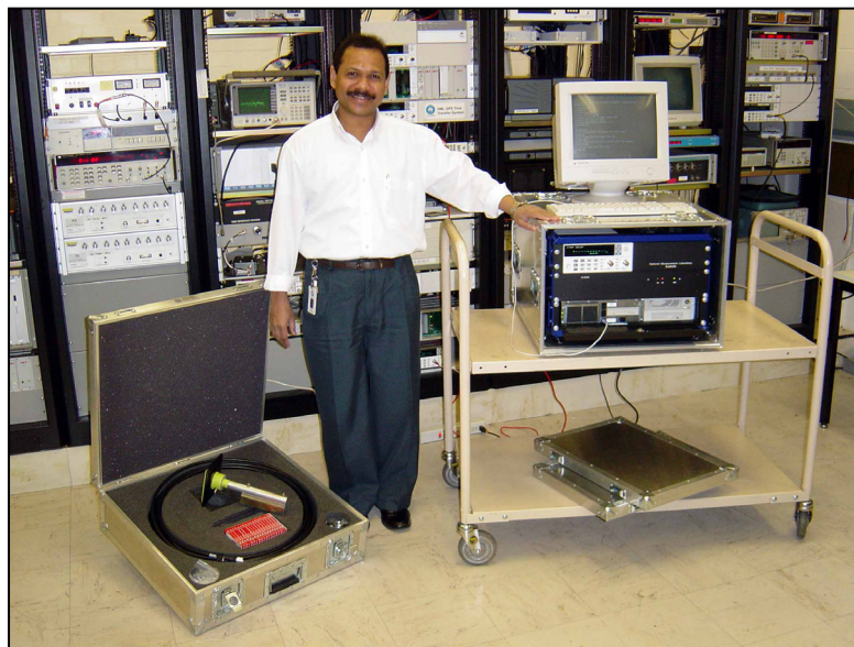
Figure 2: Anura Gajaweera of the NMI Time and Frequency group with the completed portable time-transfer system.
