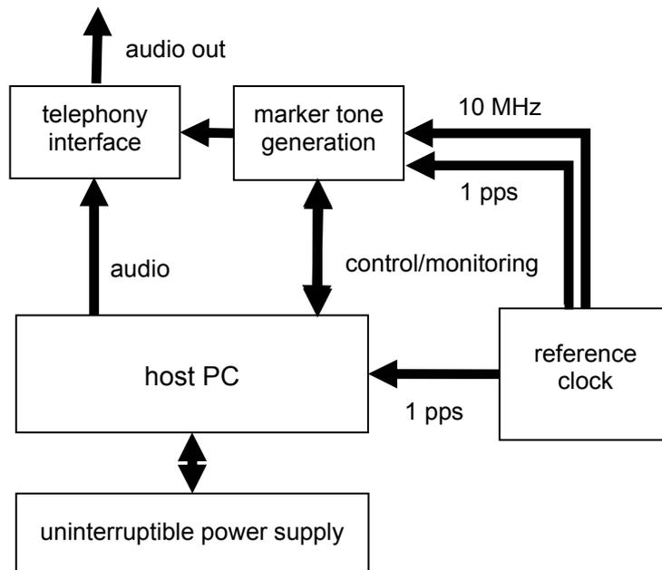
**Figure 2:** The NMI speaking clock system.
